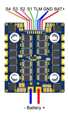
S1 – S4 – Motor Signal 1-4 TLM – Telemetry (Serial) GND – Reference Signal Ground
