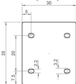
The ESC comes with a 20 mm x 20mm mounting hole layout designed for M2 and M3 screws. Original is for M2 while you can use a screw driver and force it into M3 by rotating it inside the hole carefully.
